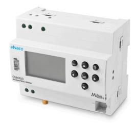
CMeX50 is a wireless M-Bus Receiver which can be easily integrated into an existing M-Bus solution or used together with Elvaco CMe Series products. The CMeX50 communicates with up to 800 wireless M-Bus meters, each one securable through individual encryption keys. CMeX50 also has an integrated M-Bus Master which enables it to drive up to 32 wired M-Bus meters. The number can be extended by using the product together with one of Elvaco's M-Bus Masters from the CMeX10-13S Series.
